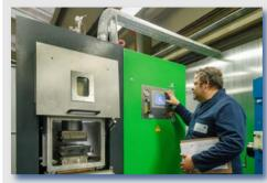
The specialist sintering press is computer controlled and so sintering cycle data from the time of pressing is recorded for every single batch to facilitate complete traceability.
