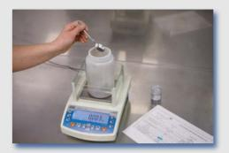
Every job is individually initiated with exact accuracy in the measurement of powders. We blend our own diamond powders and bonds, with a range of cutting characteristics, to suit all possible honing applications.
