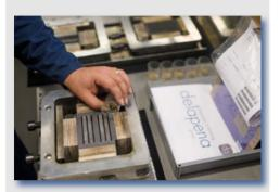
Each mould is loaded with precisely controlled powder doses. Like every stage of the process, care and attention is paid to ultimate quality.
